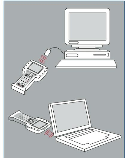
*Easy Upgrade allows communication between the 375 Field Communicator and a PC using IrDA. The IrDA port enables transfer of configuration data between the 375 and AMS Device Manager as well as upgrading of new Device Descriptions and functionality.*
